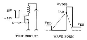
$$\begin{array}{ll} R_{\mbox{\scriptsize G}}\!=\!25\Omega \\ V_{\mbox{\scriptsize DD}}\!=\!-50\mbox{\scriptsize V}, \; L\!=\!1.44\mbox{\scriptsize mH} \end{array} \qquad E_{\mbox{\scriptsize AS}}\!=\!\frac{1}{2}\cdot L\cdot I^2\cdot (\frac{B_{\mbox{\scriptsize VDSS}}}{B_{\mbox{\scriptsize VDSS}}\!-V_{\mbox{\scriptsize DD}}}) \end{array} \label{eq:controller}$$
